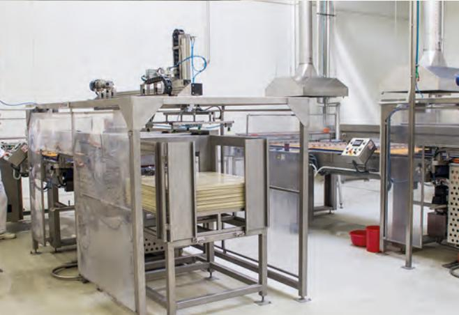
De-palletizer of autoclave baskets/autoclave baskets unloader
