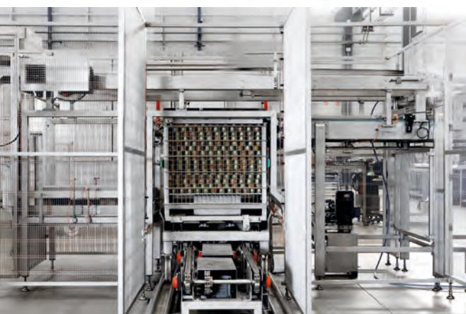
Palletizer of autoclave baskets/Autoclave basket loader
